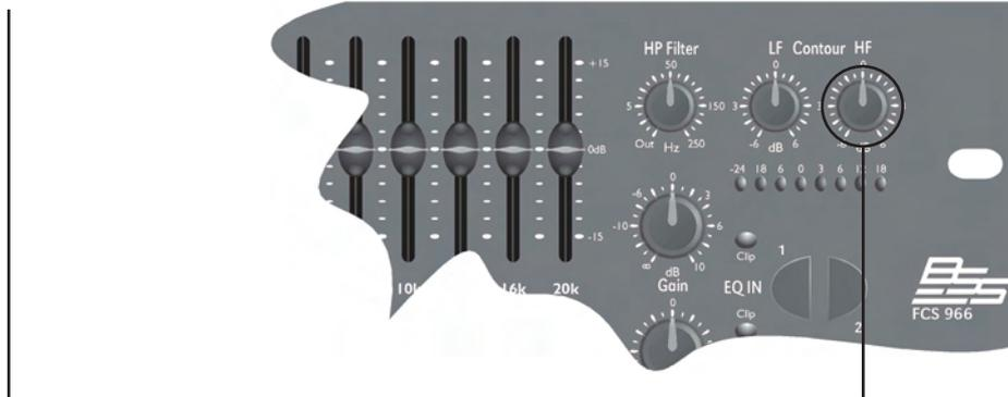
This control serves a similar purpose as the *LF contour*, but applied to higher treble frequencies. The *HF contour* control allows a subtle change to be made to the shape of the sound without affecting the previously configured main equalizer. On a creative note, the HF contour control can be used to breath 'air' into an otherwise flat sound, or remove 'brittleness' from over bright signals.
