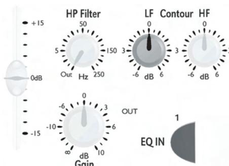
As the contour controls are gentle in operation, they are intended to be used whenever it is desired to change the tonal balance of the sound without disturbing the main equalizer settings.
