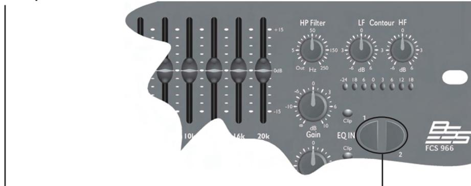
When the *eq in* switch is in the out, non illuminated position, all FCS 966 functions are bypassed and the input is connected directly to the output with a high quality relay. This condition also occurs when the power is off, and ensures that the signal is passed through the unit in the case of a power or fuse failure. When the switch is pressed, the processed signal is present on the output.
