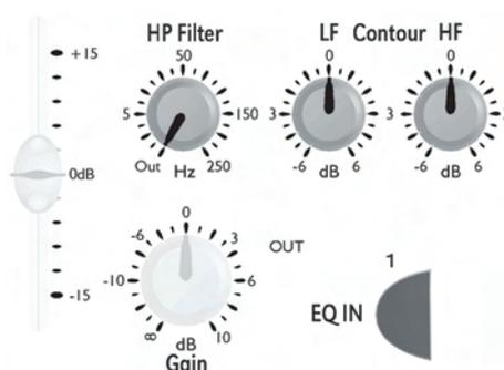
Generally when using an equalizer, you should think in terms of removing problem sounds rather than increasing the level of the good parts. The FCS 966 would normally be patched into the 'insert' point of the mixer channel carrying the signal that needs attention.
