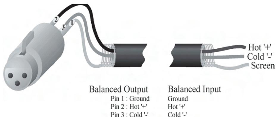
When using the FCS 966 to drive unbalanced inputs, best performance is usually obtained by connecting the FCS 966s '+' signal to the equipment signal pin and the '-' signal to the equipment shield.
