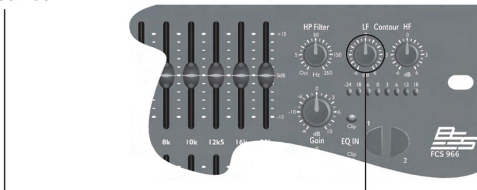
This control applies a gentle, musical, low frequency boost and cut shelving response. It works in addition to the main graphic and provides a convenient way of changing the overall sound balance without disturbing a detailed room or speaker response that has been set up on the main equalizer section. One way to think of the *LF contour* control is as a means of augmenting the main equalizer in a way that can be easily adjusted and reset.
