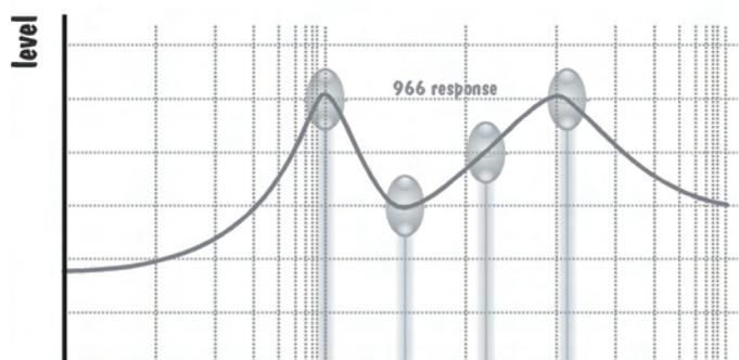
In line with its other graphic equalizers, BSS have chosen a 'constant Q' topology for the FCS 966, as this gives the best correlation between the actual slider positions and the measured response of the unit. *Figure 7.4* shows how the response of the FCS 966 follows much more closely the curve depicted by the sliders than a gyrator based graphic (*figure 7.3*). Note that the illustration is a guide only.
