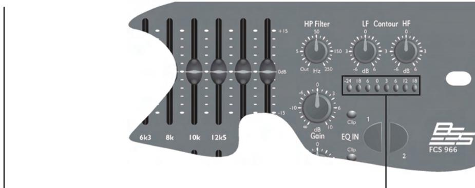
This is a peak reading RMS calibrated meter. Normally when the *eq in* buttons are depressed, it measures the signal being sent to the output connector. If the channel is bypassed (*eq in* button out), the meter reads the input signal. This allows accurate matching of the equalized and 'dry' signals using the *gain* control.
