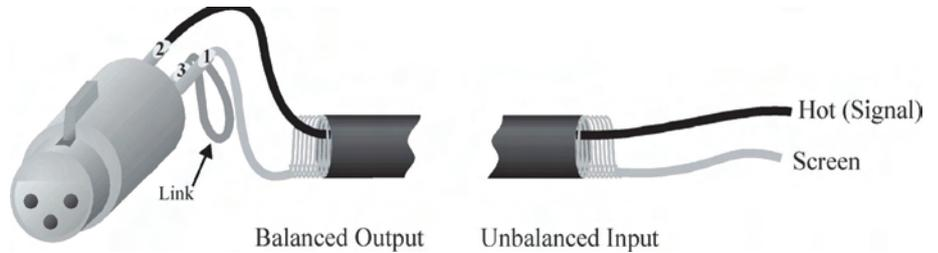
The FCS 966 shield should normally be connected to the equipment shield, preferably at the equipment end. Transformer isolated outputs are also available as a dealer fitted option.
