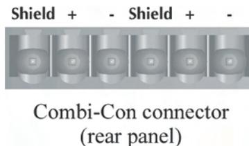
The signals are electrically identical to those on the XLR connectors. For convenience it may be desired to use individual 3 way plugs for independent connection of input and output signals wired as follows:
