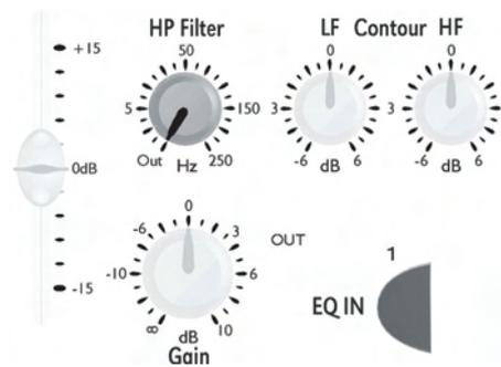
It is highly undesirable to send large amounts of low frequency energy to speaker systems that are unable to cope with it. This leads to distortion and premature overload. As the HP filter is steep, it is able to more effectively remove this energy than the main equalizer low frequency bands. In addition to
