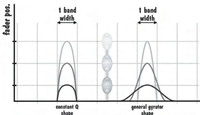
If the width varies with slider position, as it does with non constant Q equalizers, accurately summing the result from a number of sliders will be impossible except at one position, the position when the Q or width equals the space between two adjacent bands. It should be self evident that this type of operation is highly undesirable, as the effect of one slider will depend on the position of many others making the total effect unpredictable.
