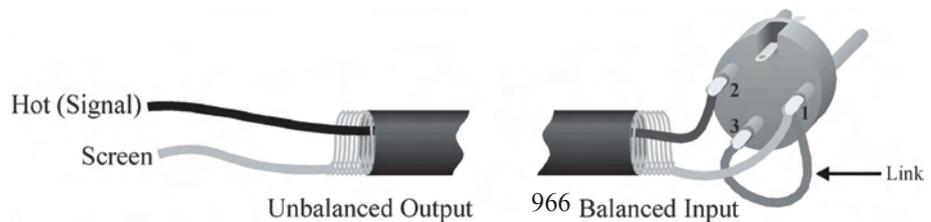
**5.2 XLR Outputs** The output signals are electronically balanced and fully floating. Full headroom is available into any load of 600 Ohms or greater. The signal 'HOT, +, or *in phase*' signal is to pin 2, the 'COLD, -, or *out of phase*' signal is to pin 3, with pin 1 being connected directly to the chassis.
