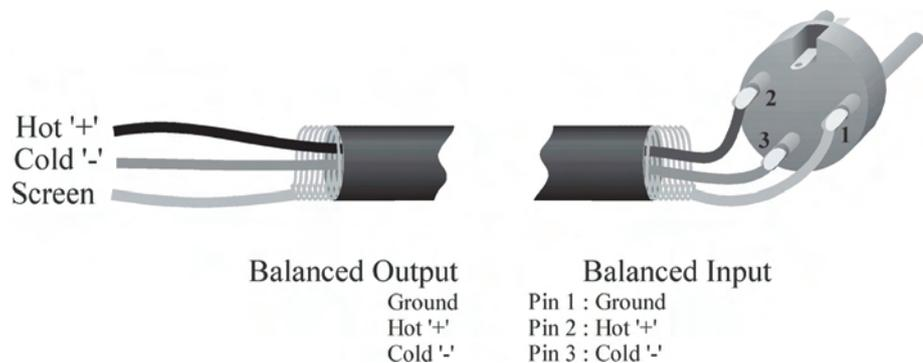
When feeding the FCS 966 from unbalanced sources, connect the signal conductor to pin 2 and the cable screen to pins **1 and 3**. Transformer isolated inputs are available as a dealer fitted option.
